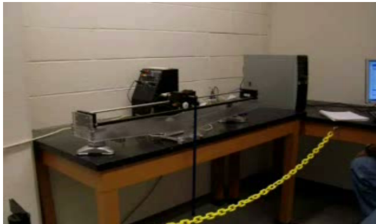
Video demonstration of the inverted pendulum experiment in our undergraduate Control Laboratory. Click for demo.
